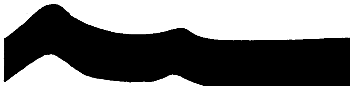
Fig. 1. Electrophoresis pattern of purified myrosinase. Ascending boundary in veronal buffer, pH 8.5, 0.1 ionic strength; time = 1 hour, 49 min. (see text for mobilities)
